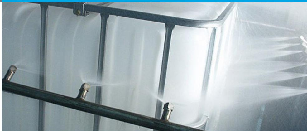
Reconditioning of an intermediate bulk container (IBC): This process circumvents the consumption of materials to produce new IBCs, thereby lowering costs. *Photo from Mauser.*
